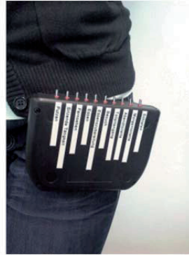
Figure 1B. Electronic protocol box worn by a healthy test volunteer. The volunteer can trip protocol the current activity by tripping the according switches.
