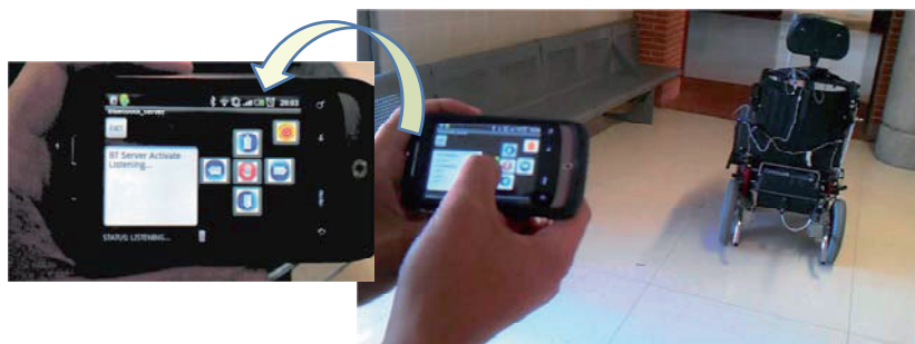
Fig. 5. Controlling the IW with a Smartphone, using the Bluetooth interface.
