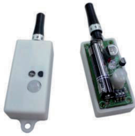
Figure 1A. One of ten 10 wireless sensor boxes with AAA battery, PIR-, light-, and temperature sensor.
