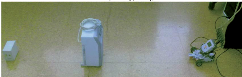
Figure 1. Mindband-controlled Lego NXT placed at the starting point of the challenge. The small white box represents the end point, whereas the larger one is the obstacle.
