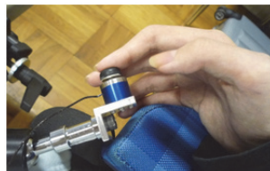
Fig. 4. Measurement of the fingertip force.
