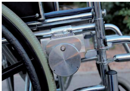
Fig. 1. Eccentric wheel solution of 1 st year team.
