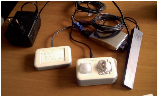
Fig. 1. The infrared sensor pair with 360 degree and directed lens-monitoring unit and wireless unit.
