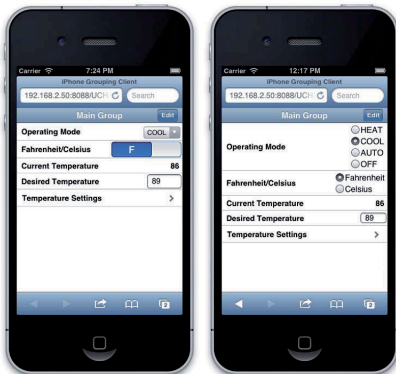
Figure 2. Two sample user interfaces for the control of a digital thermostat. (a) On the left: User interface with a drop-down menu and a toggle control for setting the operating mode and the temperature unit (Fahrenheit vs. Celsius). (b) On the right: Variation of (a) with sets of radio buttons in place of the drop-down menu and the toggle button. Notes: (1) Although shown as rendered on an iPhone here, the user interfaces generated by GenURC run on any Web-based platform, including desktop computers. (2) A textual description is available for each of the screen shots.
