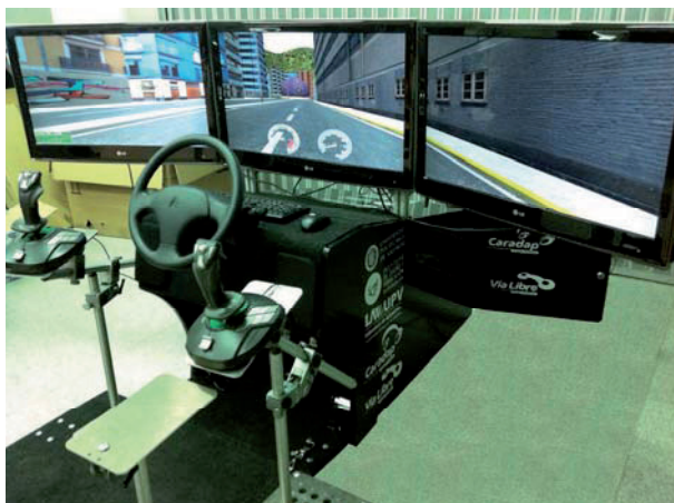
Fig. 1. Layout of Driving Simulator “J4D” (Joystick-for-Driving).
