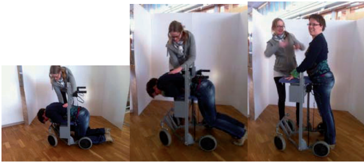
Figure 3. The lifting process.
