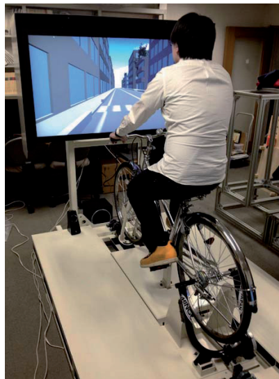
Fig. 2. Appearance of the Developed Bicycle Simulator System.
